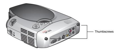
3. Carefully pull the video adapter straight out and away from the projector body.
